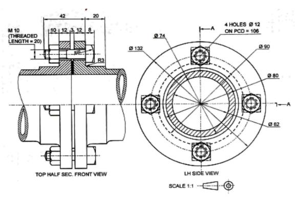
ASSEMBLY OF A FLANGED PIPE JOINT
